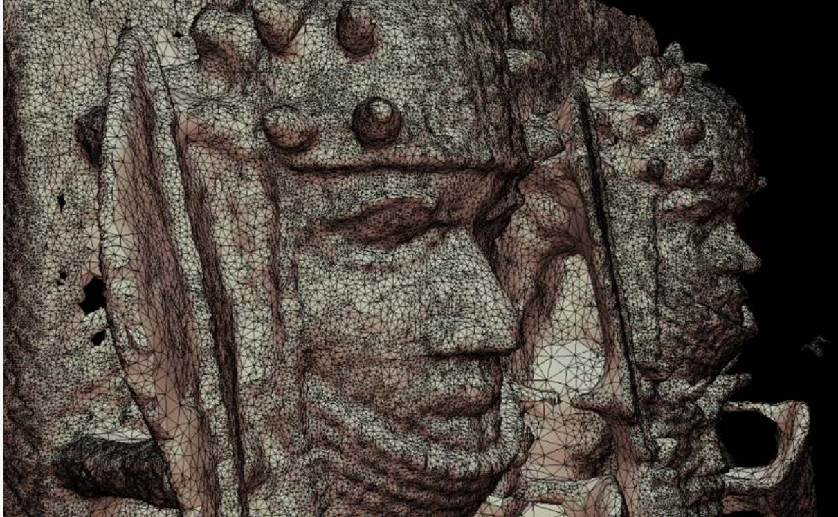
Figure 6 – Combined mesh and wireframe of an output model created through photogrammetry. Credit: MOWAA Digital Team
